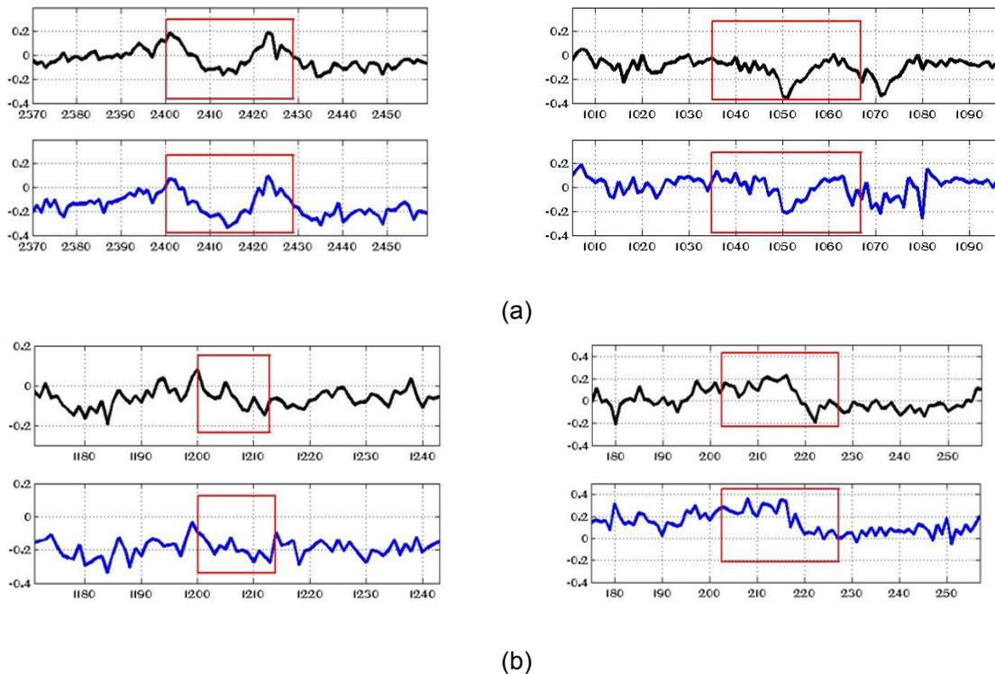
**Figure 11 Comparisons of (a) a scenario when both the referenced and the reoriented accelerometers were correctly detected the events, and (b) a scenario when the reoriented accelerometer detected the event, but the referenced acceleration did not. The  $y$  – accelerations are shown on the left, and  $x$  – accelerations are shown on the right**
