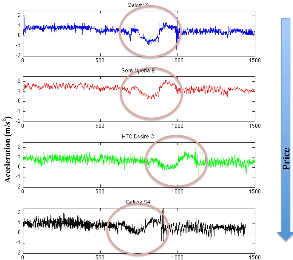
Figure 19 Raw Accelerometer Data of 4 Smartphones
