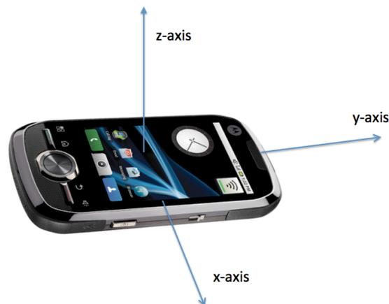
**Figure 1: 3-axis Accelerometer**
