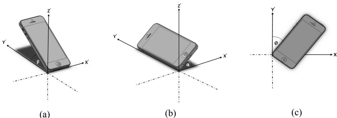
**Figure 9 An illustration of angular rotations around (a) the  $x'$  axis, (b)  $y'$  axis, and (c)  $z'$  axis**
