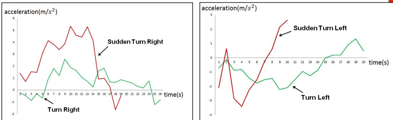
**Figure 6 Example of raw data collected from accelerometer sensors illustrating turning events**
