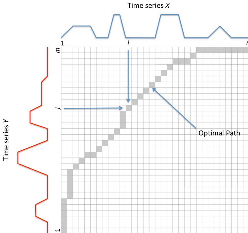
**Figure 2: Dynamic Time Warping Grid**
