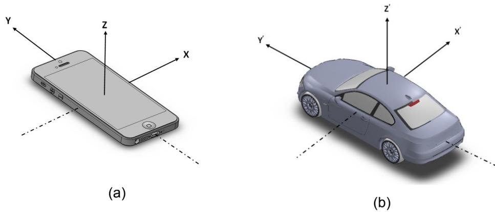
**Figure 8 (a) The orientation of a smartphone described by  $(x, y, z)$  coordinate system, and (b) the direction of the vehicle movement given by  $(x', y', z')$  coordinate system**
