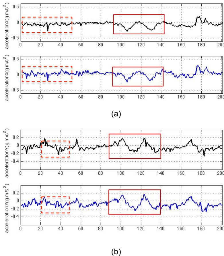
**Figure 10 Comparisons of (a)  $x$  – acceleration and (b)  $y$  – acceleration between the referenced accelerometer (in black), and the automatic reoriented accelerometer (in blue).**
