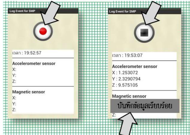
Figure 14 Sensory data collector application
